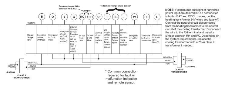
NOTE ⊕: Connection for Call for Service diagnostic indicator compatible with mechanical or electronic condenser control with Comfort Alert™.
