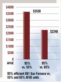
This chart depicts potential energy savings you can expect from the G61 furnace, versus older furnaces with lower efficiency ratings. Criteria used in this example are 2,000 full-load heating hours, with a 60,000 Btuh heating design load and \$1.281 ccf for gas. Your actual savings may vary, depending on the weather patterns in your local area, local fuel rates and your individual lifestyla
