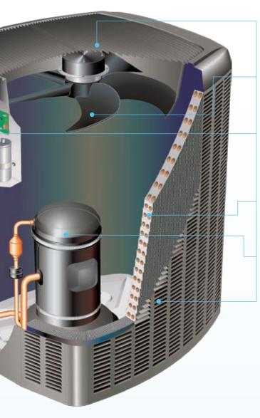
SilentComfort<sup>™</sup> Fan Grille – Uses patentpending, vortex-suppression technology to reduce sound of airflow exiting unit, providing a quieter environment outside your home.
