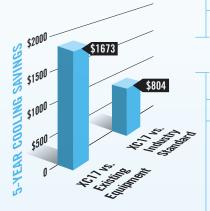
SEER stands for "Seasonal Energy Efficiency Ratio" and is a measure of the cooling efficiency of air conditioners. The higher the SEER, the greater your energy savings. Typical SEER ratings start at 13.00, but the XC17 carries ratings as high as 18.00.
