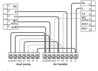
Stage 2 compressor and auxiliary heat **Note:** Do not jumper Rc or Rh, ecobee3 does this automatically. R can go into either Rc or Rh terminals on your ecobee3.
