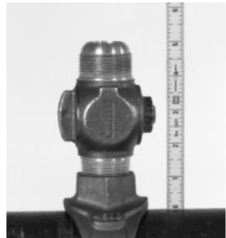
Figure 8 – Measuring valve standoff distance
