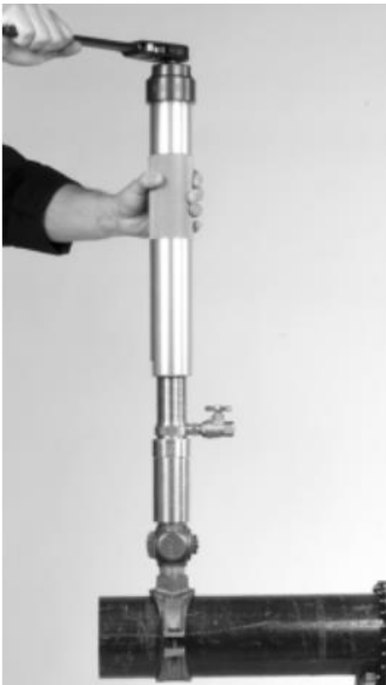
Figure 12 – Pivot of hand on ratchet and other hand on tool
