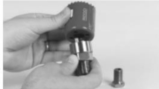
Figure 4a – Installation of cutter on large hole saw arbor
