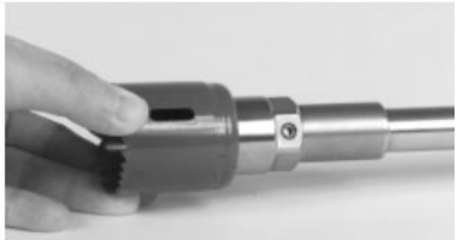
Figure 3a – Installation of large hole saw adapter
